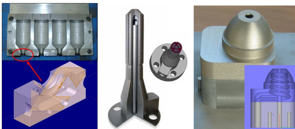
Figure 7: Cooled inserts for tooling. (a) left: for the necks of bottles in a blow mould. (b) middle: core for cooling the injection point of a mould. (c) right: hybrid core with conformal cooling built on top of machined base. Courtesy of SIG Blowtec, Es-Tec, DemoCenter, LBC.
