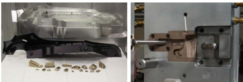
Figure 6: (a) left: machined aluminium tool and DMLS inserts. (b) right: tool with DMLS sliders and guides in different materials. Courtesy of General Pattern, Linear.
