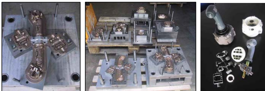
Figure 2: Series production of a joystick for a construction vehicle. Left: injection mould (core side) for two components. Middle: four completed tools. Right: moulded components and assembled joystick. Courtesy of FIT GmbH
