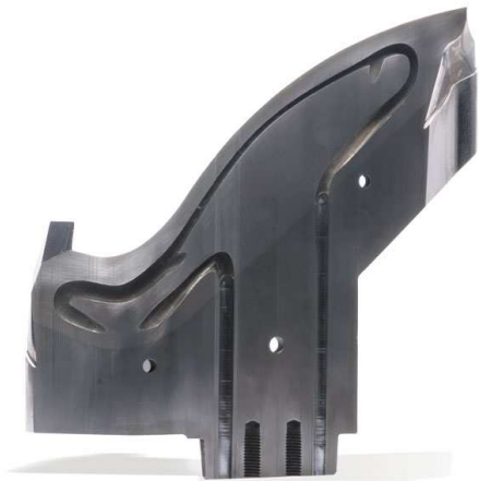
Hybrid insert for injection moulding with cooling channels
