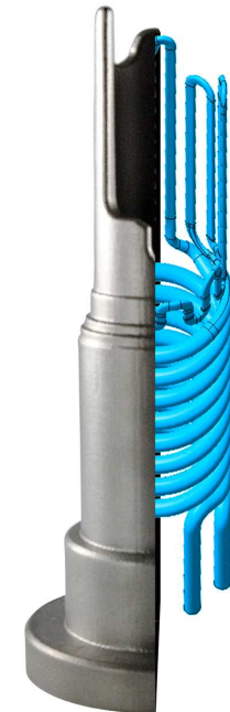
Tool insert for injection moulding with conformal cooling
