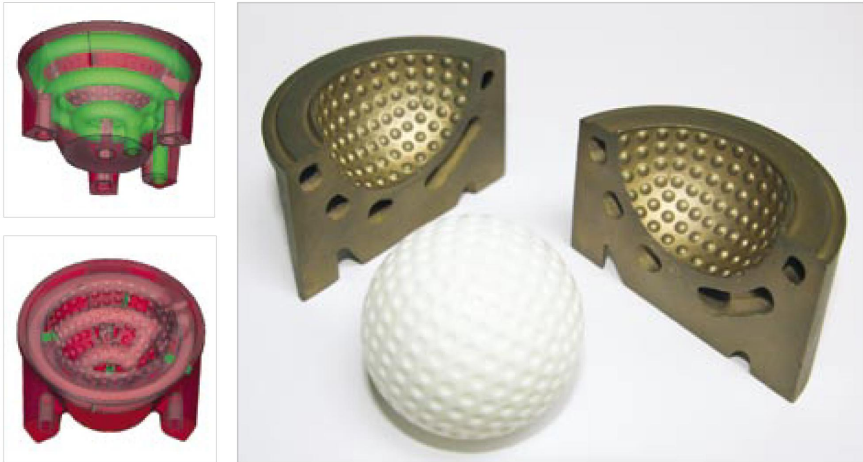
Figure 4 Golf Ball blow-mould Left: Conformal cooling Middle: Venting channels (Green) Right: DirectTool cavity Courtesy: Es-Tec, DemoCenter
